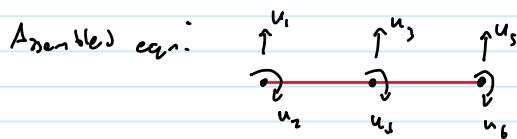
$$\frac{\sum EI}{L^3} \begin{bmatrix} 6 & -3L & -6 & -3L & 0 & 0 \\ -3L & 2L^2 & 3L & L^2 & 0 & 0 \\ -6 & 3L & 6+6 & 3L-2L & -6 & -3L \\ -3L & L^2 & 3L-2L & 2L^2+2L^2 & 3L & L^2 \\ 0 & 0 & -6 & 3L & 6 & 3L \\ 0 & 0 & -2L & L^2 & 3L & 2L^2 \end{bmatrix} \begin{Bmatrix} u_1 \\ u_2 \\ u_3 \\ u_4 \\ u_5 \\ u_6 \end{Bmatrix} = \frac{q_0 L}{12} \begin{Bmatrix} 6 \\ -L \\ 6 \\ 1 \\ 0 \\ 0 \end{Bmatrix} + \begin{Bmatrix} Q'_1 \\ Q'_2 \\ Q'_3 + Q'_4 \\ Q'_5 + Q'_6 \\ Q'_7 \\ Q'_8 \end{Bmatrix}$$
