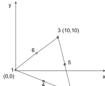
$$\begin{aligned} \iint_A \psi_1^2 dA &= \iint_A [L_1(2L_1 - 1)]^2 dA \\ &= 4L_1^4 + L_1^2 - 4L_1^3 dA \end{aligned}$$
